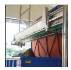
FSM conveyors are used to convey solid matter and are available in two main designs – as a screw conveyor with self-supporting central shaft or as spiral conveyor without central shaft.
